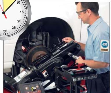
**Step 3: Adjust cut depth and machine rotor with on-the-fly optimum speed.**
