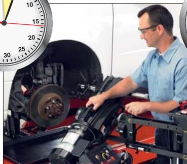
**Step 1: Attach adaptor and lathe...**
