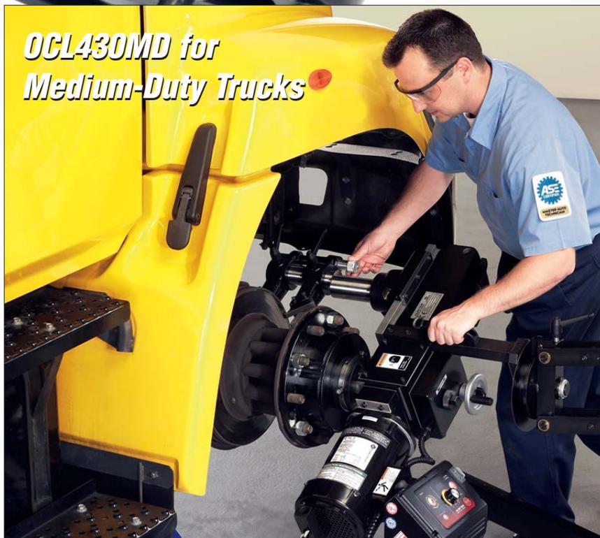
**Panel display reads right side up no matter which way the lathe is rotated. Adjustment controls can be accessed easily from outside the fender well.**
