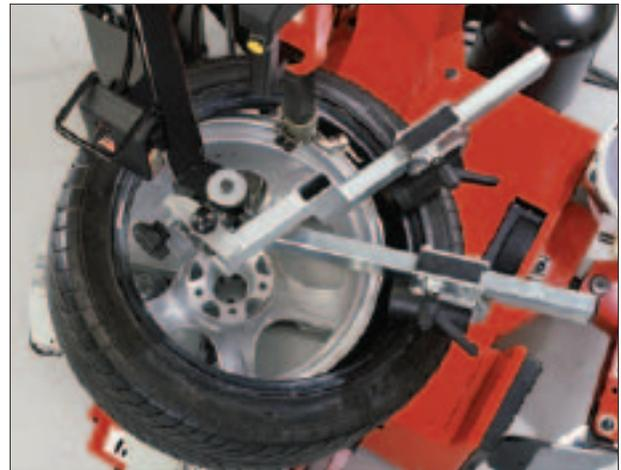
**When combined with the rotating arm, the fixed bead press arm adds additional bead pressing force to service the most extreme low-profile tires and deep drop-center alloy wheels.**
