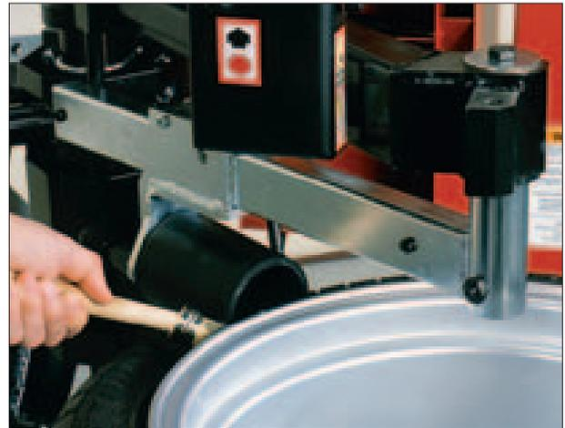
**Tapered rollers assist in bead lubrication and bead lever placement to ease demounting.**
