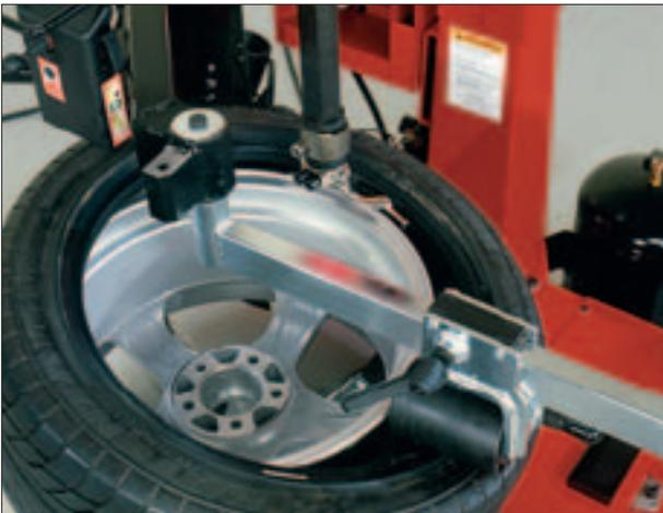
**A single bead press roller with rotating arm can quickly be used for mounting and demounting stiff sidewall tires. The roller may be locked to hold the tire sidewall, which maintains traction during the mounting sequence.**
